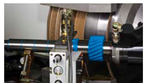
Angled infeed grinding
